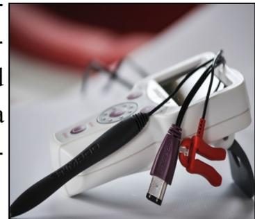
Its stimulation probe is designed to direct the current to a particular nerve or region, such as a joint or muscle. It enables practitioners to evaluate the treatment progress of damaged nerves.
